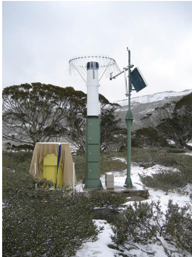
A pedestal pluviometer prior to the installation of its protective wind fence.
